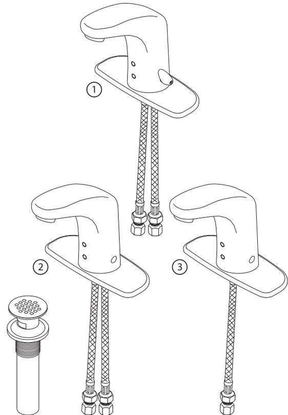
housing. Place faucet supply(s) through wash basin and secure using wing fixing plate and nuts from single mount kit.
